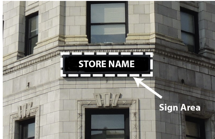
Figure 710-C: Illustration of computing the sign area for wall signs with a background panel or cabinet.
