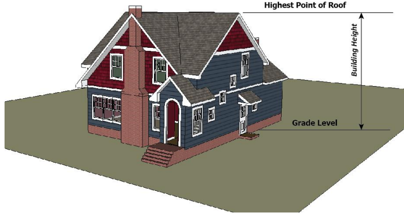
Figure 702-H: Measurement of building or structure height
